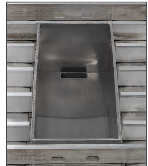
The Bow Anchor Locker compartment is built in to the frame of the HTH and the In-tube Storage compartment is even deeper.
