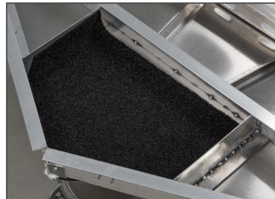
The Bow Anchor Locker compartment is built in to the frame of the HTH and the In-tube Storage compartment is even deeper.
