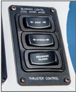
Intuitive Thruster System Control
