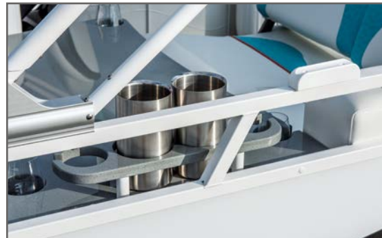
White .090 Square Aluminum Textured Powder Coated Rails
